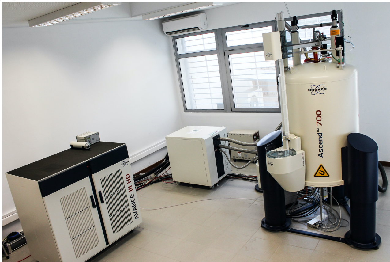
High Definition 700MHz NMR, 4channels ( ^1\text{H}/^2\text{H}/^{13}\text{C}/^{15}\text{N} ) & TCI Cryoprobe Department of Pharmacy
